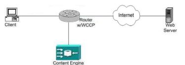
Refer to the exhibit. The exhibit shows a Content Engine with WCCP enabled between the Content Engine and the router. The Client browser is configured for direct connection to the Internet.
