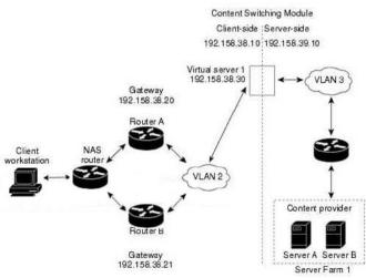
You configure single subnet (bridge) mode by assigning the same IP address to the CSM client and server VLANs. In bridge mode the client does not point it's Default Gateway to the CSM. To configure content switching for the single subnet (bridge) mode, perform this task:
