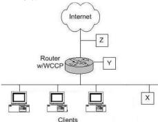
Refer to the exhibit. The network diagram has a WCCP enabled router. Where should the Content Engine be placed to minimize the load on the router for caching
