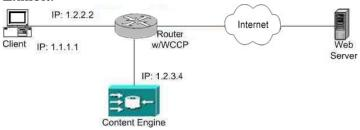
Refer to the exhibit. The exhibit shows a Content Engine with WCCP enabled between the Content Engine and the router. The Client browser is configured with an HTTP proxy address of 1.2.3.4.
